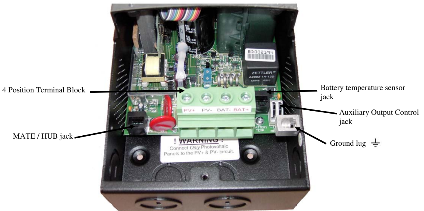
Figure1. MX60 charge controller wiring compartment
